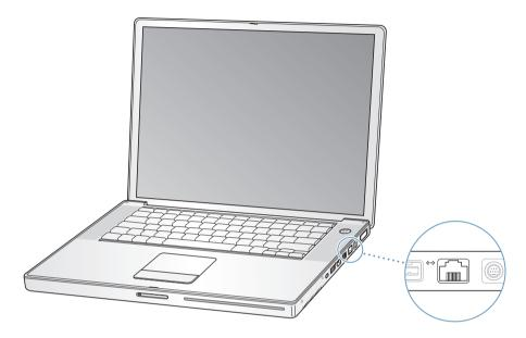
Connecting to a network gives you access to other computers. You may be able to store and retrieve information; use network printers, modems, and email; or connect to the Internet. You can also use Ethernet to share files between two computers or set up a small network. The Ethernet port on your PowerBook automatically detects other Ethernet devices. You don't need an Ethernet crossover cable when connecting to other Ethernet devices.
